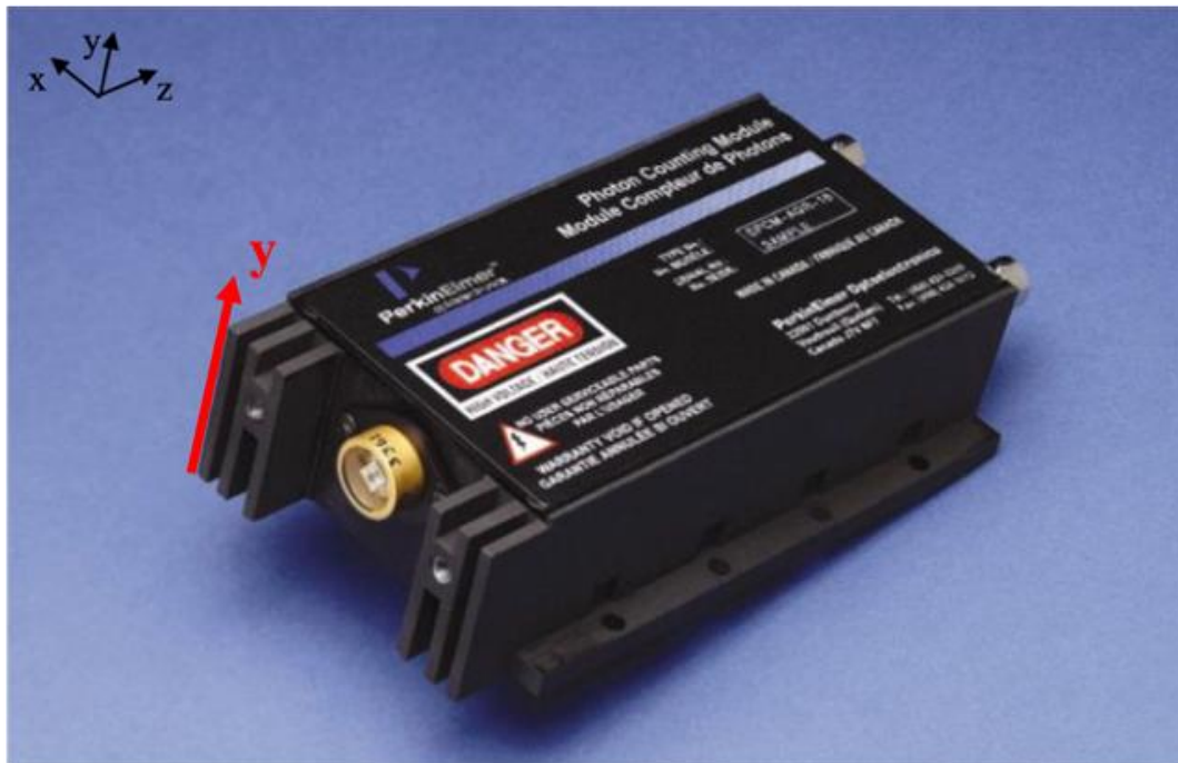
Fig. 4. The coordinates for non-uniformity scanning
