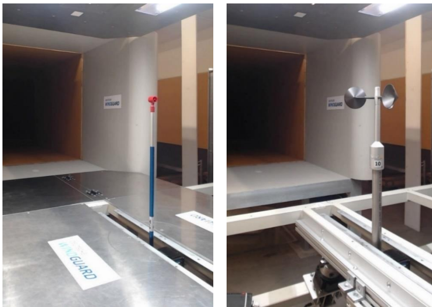
Fig. 4.4 Examples of the installations with open test section boundary. The installation on the left is used for TSR MINI and TSR MACRO anemometers. The installation on the right (larger surface uncovered) is used for the RM Young Gill Propeller and all the cup anemometers with Thies FCA mounting.
