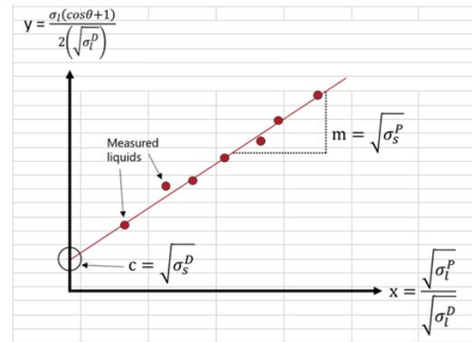
Use of OWRK Model for the calculation of surface energy using 3 contact angle measurements Of ultrapure water, ethylene glycol and diiodomethane
