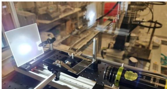
Measurement of contact angle
