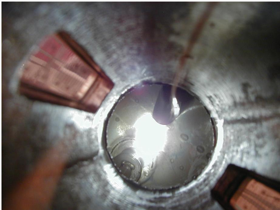
Fig. 6 - Insight into the TS cavity with bottom plate and displacer
