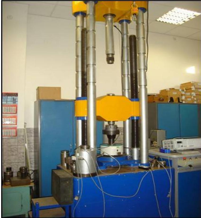
Figure 2. 1 MN INM Comparator type Force Standard Machine
