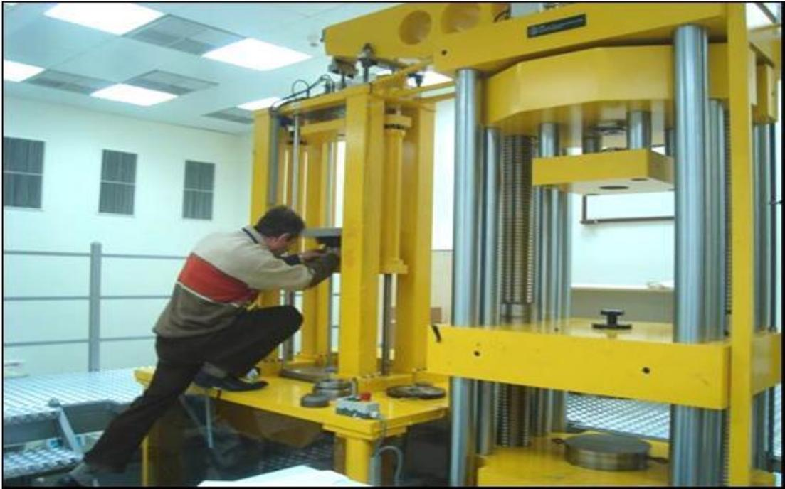
Figure 1. 110/1100 kN Lever Amplification Force Standard Machine of UME
