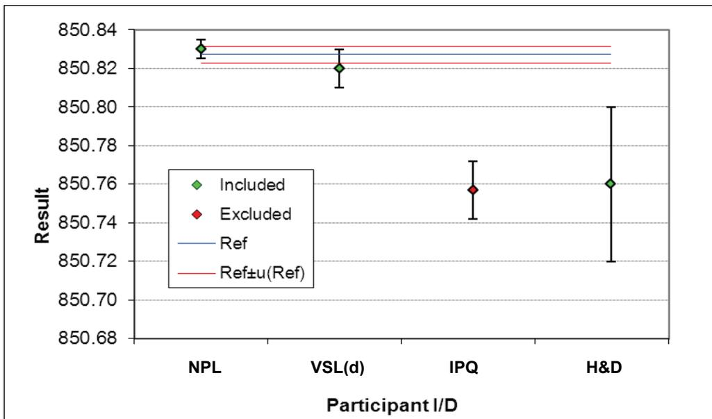
Figure 6d Amended results of the comparison for the Vitrea 100 oil at 70 °C.
