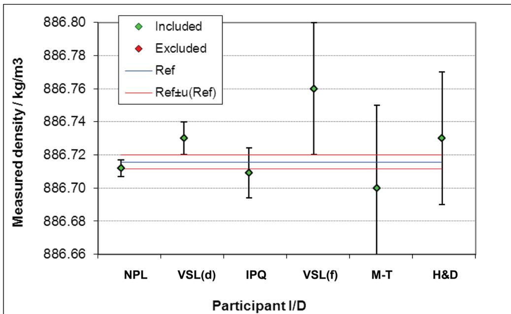
Figure 5b Results of the comparison for the Vitrea 220 oil at 20 °C
