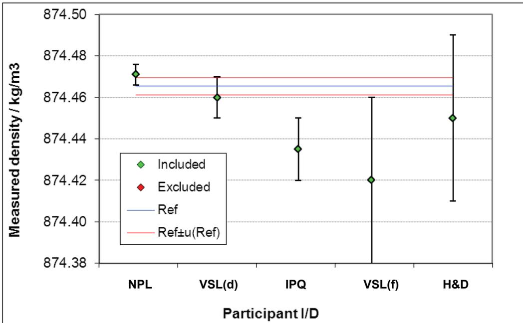
Figure 5c Results of the comparison for the Vitrea 220 oil at 40 °C
