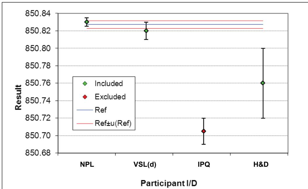
Figure 4d Results of the comparison for the Vitrea 100 oil at 70 °C
