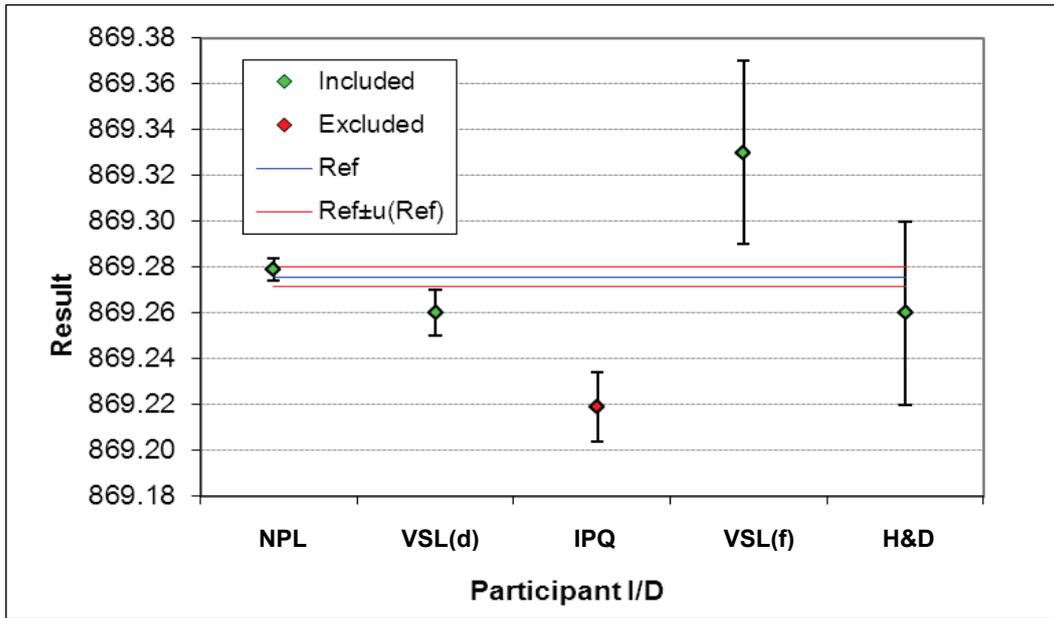
Figure 4c Results of the comparison for the Vitrea 100 oil at 40 °C
