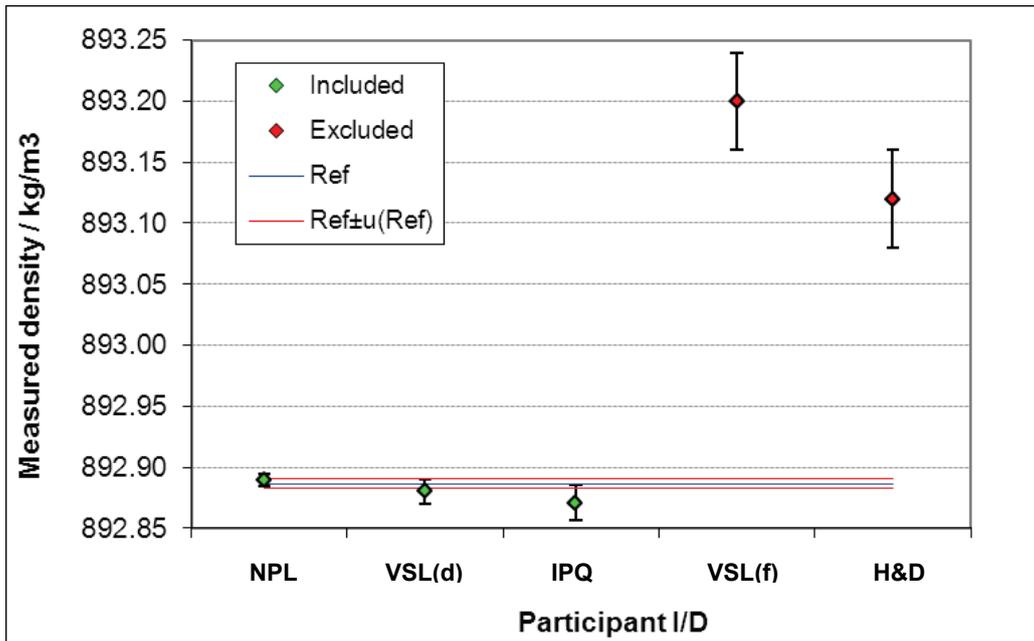
Figure 5a Results of the comparison for the Vitrea 220 oil at 10 °C
