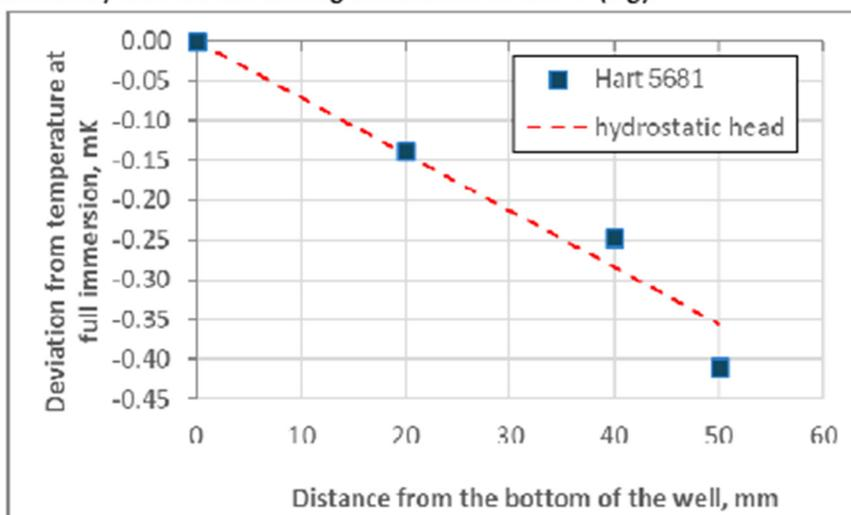
Heat-flux (immersion) test results during realization of the FP(Ar):
