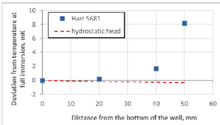
Heat-flux (immersion) test results during realization of the TPW:
