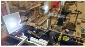
Measurement of contact angle
