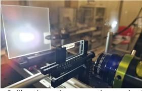
Calibration using an angle standard
