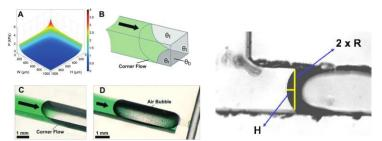
Contact angle on a surface and in a channel
