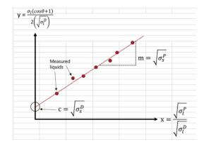
Use of OWRK Model for the calculation of surface energy using 3 contact angle measurements Of ultrapure water, ethylene glycol and diiodomethane
