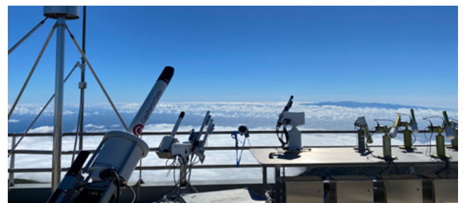
The BTS-Solar array spectroradiometer deployed at the 19ENV04 EMPIR MAPP field campaign at Izaña, Tenerife, September 2022
