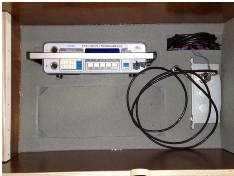
Figure 3.3 The transport case opened; location of mains cable, ASL F250 and HMT335 (with the probe).
