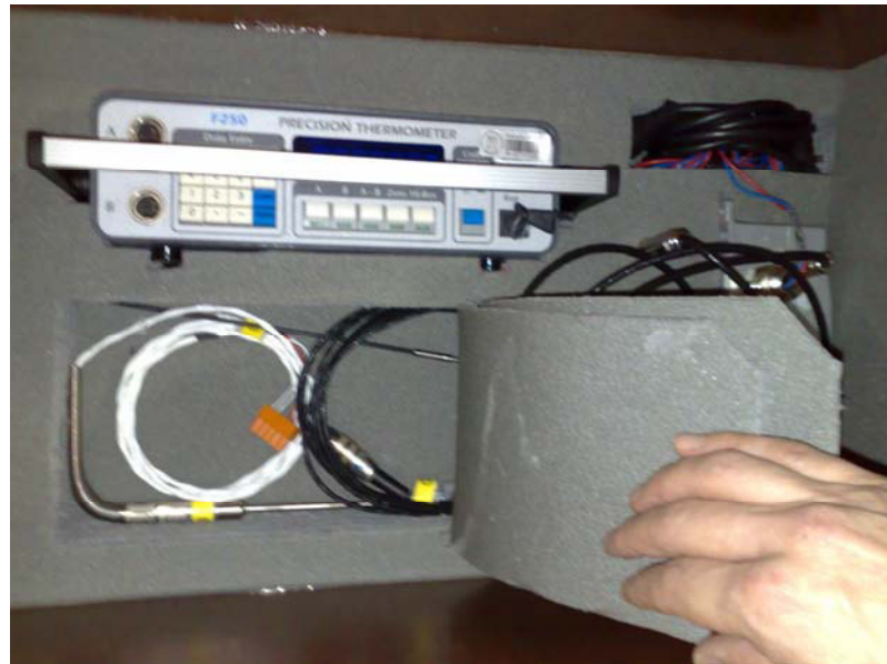
Figure 3.4 The transport case opened; location of PRTs.
