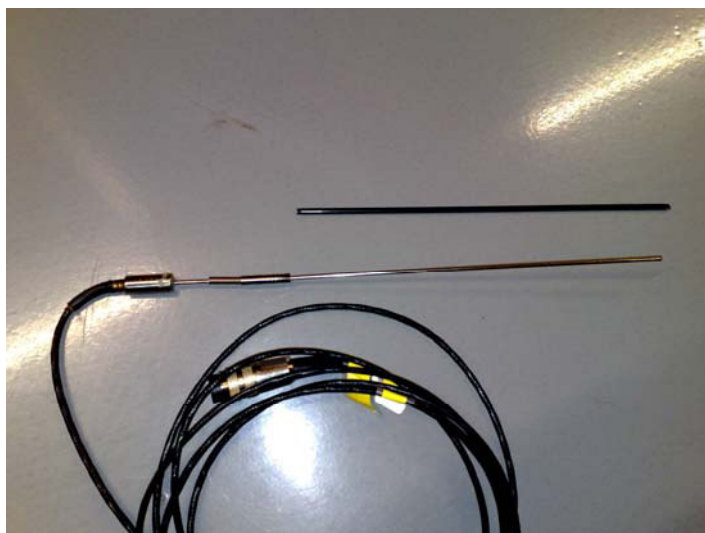
Figure 3.1 The probe A with its cover and when pulled apart from its handle part.
