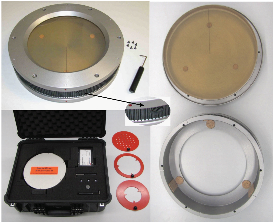
Figure 1. Specimen mounted in the housing (top, left) and inserted in the transport case (bottom, left) with environmental recording instrument and masks. The insert in the center shows the plastic screw for the transport lock. The housing consists of a base plate with three support pads for the horizontal orientation (top, right) and a cover (bottom, right). Inside the cover, three rectangular cork pads are fixed which support the specimen in the vertical orientation. The three round cork pads are only for protecting the specimen.
