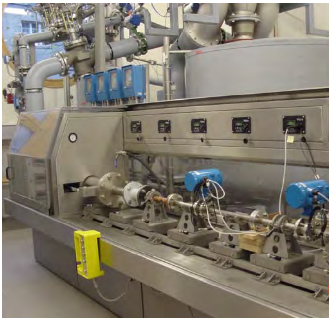
Fig. 2: Installation of the two meters in the test rig of the BEV
