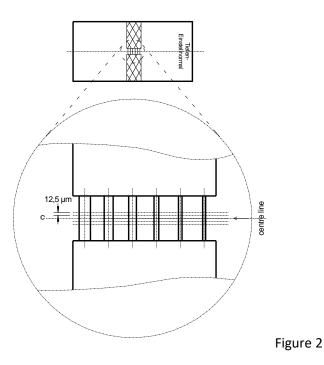
For stylus instruments the speed of traverse should be **slower than 0.2 mm/s**. The determination of the depth of the grooves **d** must be carried out according to the procedure described in ISO 5436-1. If this cannot be measured, calculate **Pt** according to ISO 4287 **for an approximation**. The evaluation length
