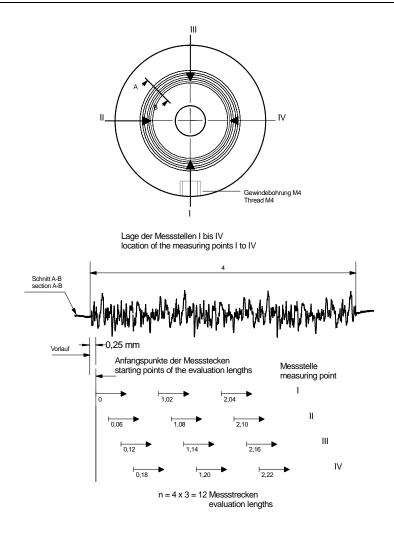
Figure 7 - The area of measurement shows the starting points and traversing direction of the respective evaluation lengths of **1.25 mm**.
