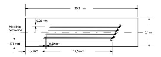
Figure 5- The area of measurement shows the starting points of the respective evaluation lengths of **12.5 mm**.
