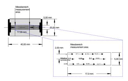
Figure 6 - The area of measurement shows the starting points and traversing direction of the respective traversing lengths of **5.6 mm**.
