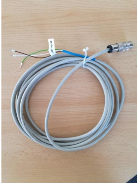
Fig. 21 The cable for the anemometer Thies
