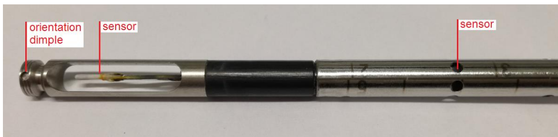
Fig. 23 The end-part of the anemometer Airflow containing the velocity, temperature and humidity sensors
