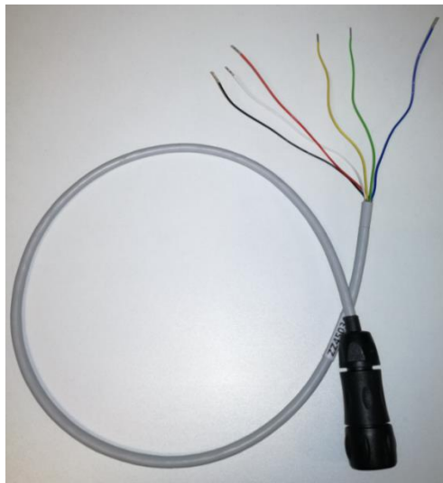
Fig. 16 Cable for the anemometer Vaisala
