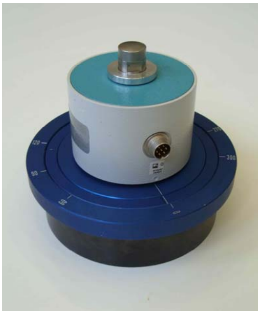
Fig. 2: Force transducer mounted on the auxiliary plate
