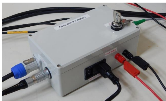
Figure 10: Electronic box 2 (alternative junction) for power supply of both transfer meters and auto zero setting for coriolis meter
