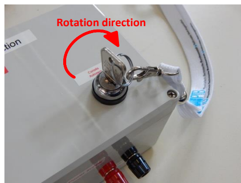
Figure A 1: Electronic box 2 and the plugged key for setting Auto zero of coriolis meter
