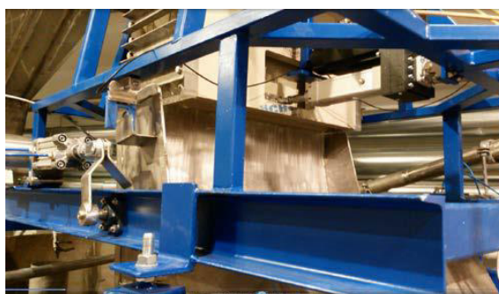
Water flow through diverter
