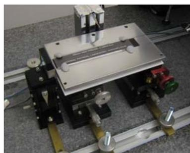
For K7, the NRC Airy-point fixtures were not suited to directly support the 100 mm scale on its Airy points, and so it was simply laid flat on the invar platform support and fixed with plastic putty at its sides.
