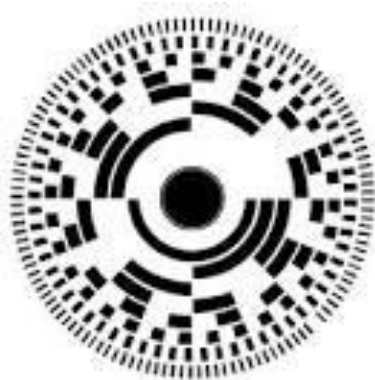
Figure 2.1.1: Coded disc of an absolute encoder. Courtesy of solo-labs.com. ( https://www.solo-labs.com/rotary-encoders-understanding-practical-implementation/ )
