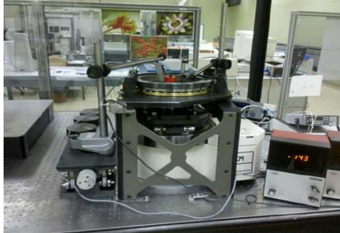
Figure 5.3.1 Example of a device at CEM to align the test encoder with the reference encoder
