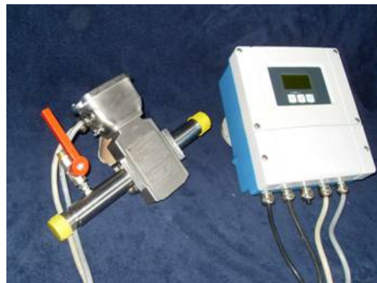
Fig. 2 Endress and Hauser - Magnetic inductive volume flow meter; Pipe size Ø 2 mm
