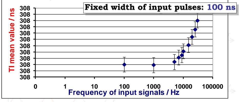
Up to about 5 kHz of input signal, there is no observed change of Time Interval between output signals of InLambda standard
