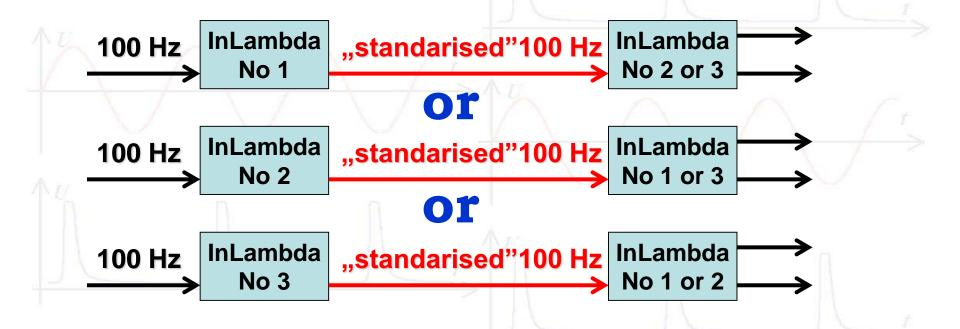
The problem of the change of Time Interval between output signals when the slope of input signals changes can be reduced by the usage of the Start output signal of one InLambda standard to the input of the other InLambda standard beeing measured.
