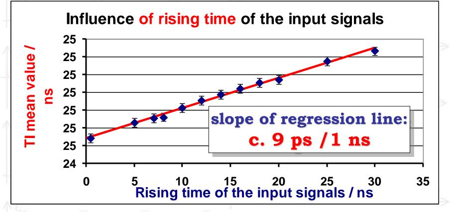
There is observed the change of Time Interval between output signals when the slope of input signals changes
