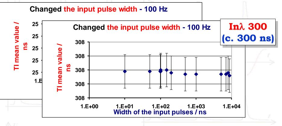
At frequency 100 Hz of input signal, there is no observed change of Time Interval between output signals at least up to 9 ms of the width of the pulses.
