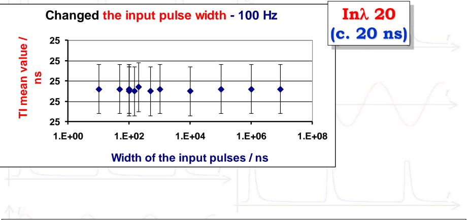
At frequency 100 Hz of input signal, there is no observed change of Time Interval between output signals at least up to 9 ms of the width of the pulses.
