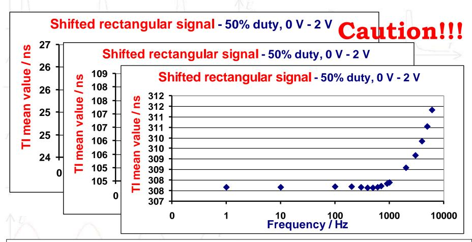
Up to about 200 Hz of the shifted rectangular input signals (duty cycle 50%, low level 0 V, high level 2 V), there is no observed change of Time Interval between output signals.
