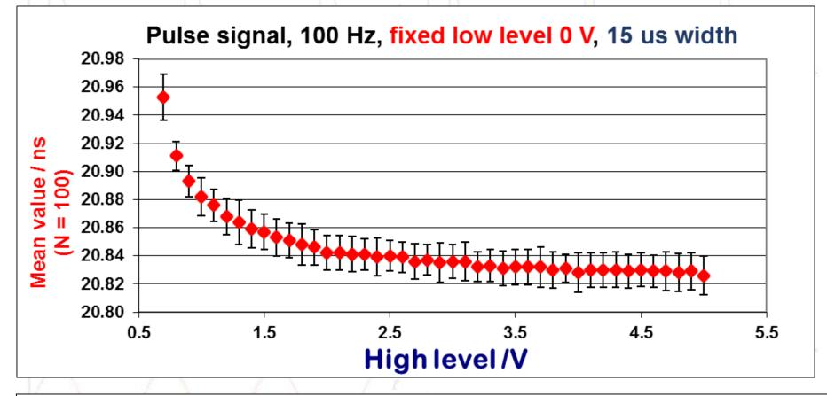
From about 2 V of the high level of input signal, there is slow change of Time Interval between output signals with increasing the high level of input signal.
