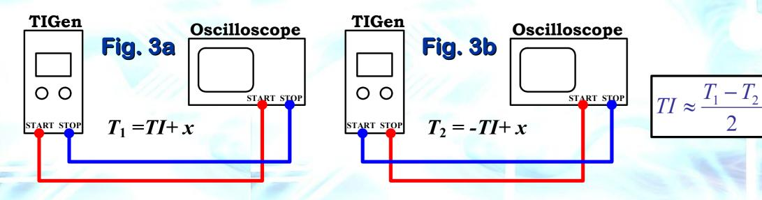
I. TWO CONSEQUTIVE SERIES OF MEASUREMENTS: IN NORMAL CONFIGURATION (Fig. 3a) AND WITH REPLACED THE CABLES BETWEEN THE START AND STOP OUTPUTS OF TIGEN (Fig. 3b)
