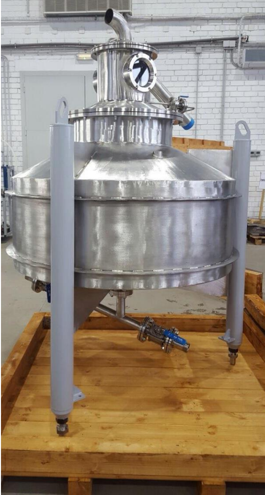
figure 1: proving tank of VNIIM
