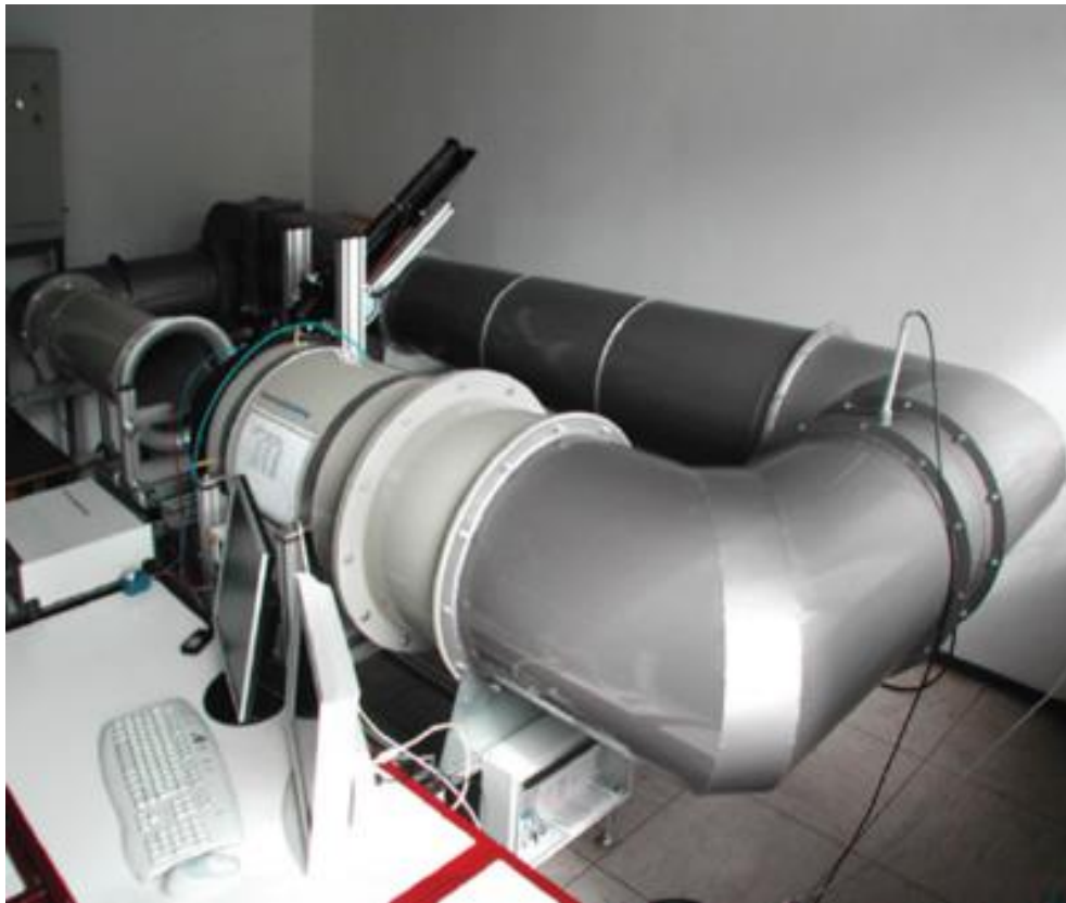
Fig. A.9 Wind tunnel of WE, nozzle diameter 255 mm
