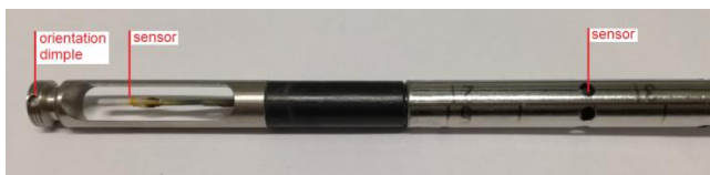
Fig. 2.9 The sensor part of the anemometer Airflow
