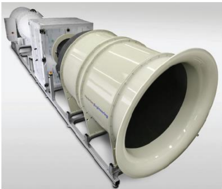
Fig. A.2 Wind tunnel WE, nozzle diameter 800 mm
