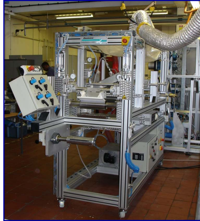
Electro-spinning device for making nanowires & fibres (e.g. bone regeneration scaffolds)
