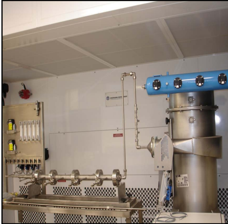
Aerosol reactor for manufacturing Inorganic core-shell nanoparticles for energy applications.
