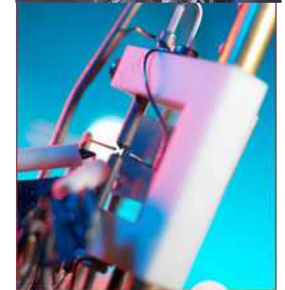
The ovens and electrodes of the NPL strontium ion end-cap trap.
