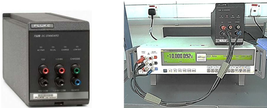
Fig. 2: Direct Measurement of 10V DC using Fluke-732B Ref. St.
