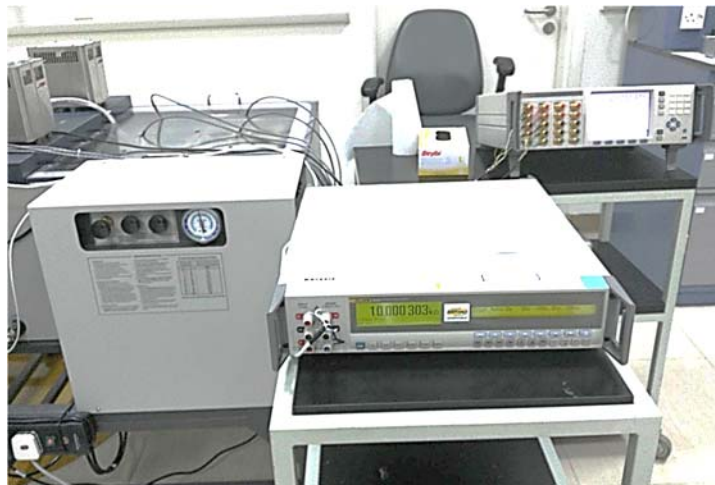
Fig. 5: Direct Method for calibration of DC Resistance
