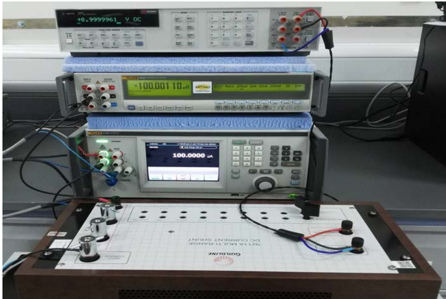
Fig. 4: In-Direct Method for calibration of DC Currents
