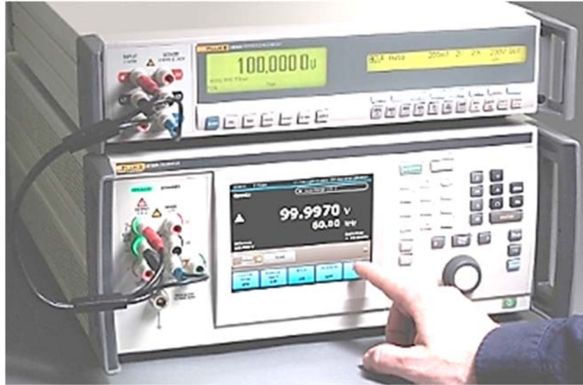
Fig. 6: Direct Measurement of 100 mV @ 55 Hz and 1 kHz using Calibrator Fluke-5730A
