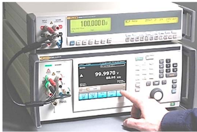
Fig. 3: Direct Method for calibration of 100 mV DC
