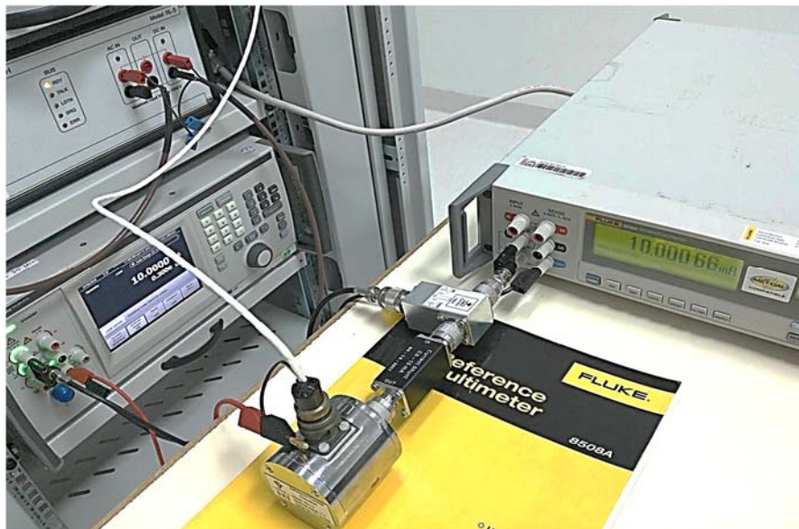
Fig. 7: In-Direct Method for calibration of AC Currents
