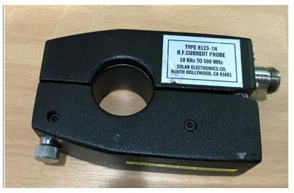
Figure 1. The photo of the travelling standard.
