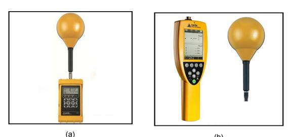
(a) (b) **Figure 1**. The photo of the travelling standards, a) ELT 400, b) HF3061 with NBM-550
