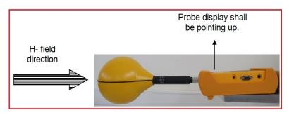
Figure 2. The position of magnetic field probe during comparison measurements
