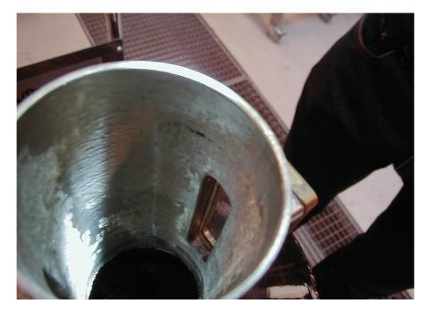
Fig. 5 - Inner surface of the TS neck
