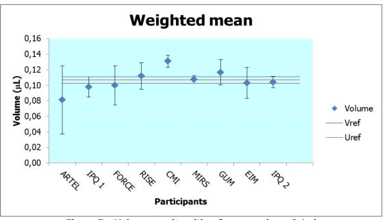
Figure 7 – Volume results with reference value – 0,1  $\mu l$
