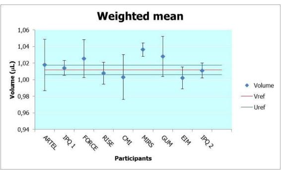
Figure 6 – Volume results with reference value – 1  $\mu$ l
