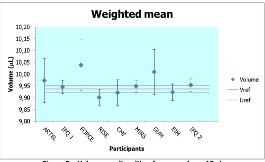
Figure 5 – Volume results with reference value – 10  $\mu l$
