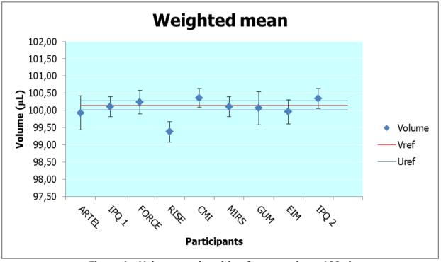
Figure 4 – Volume results with reference value – 100  $\mu l$
