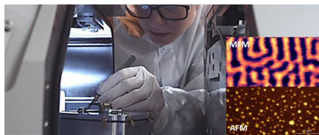
Measurement of magnetic properties with an integrated NenoVision AFM system into SEM
