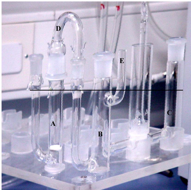
Fig. 1. Harned cell vessel. The horizontal line indicates the cell vessel immersion level.
