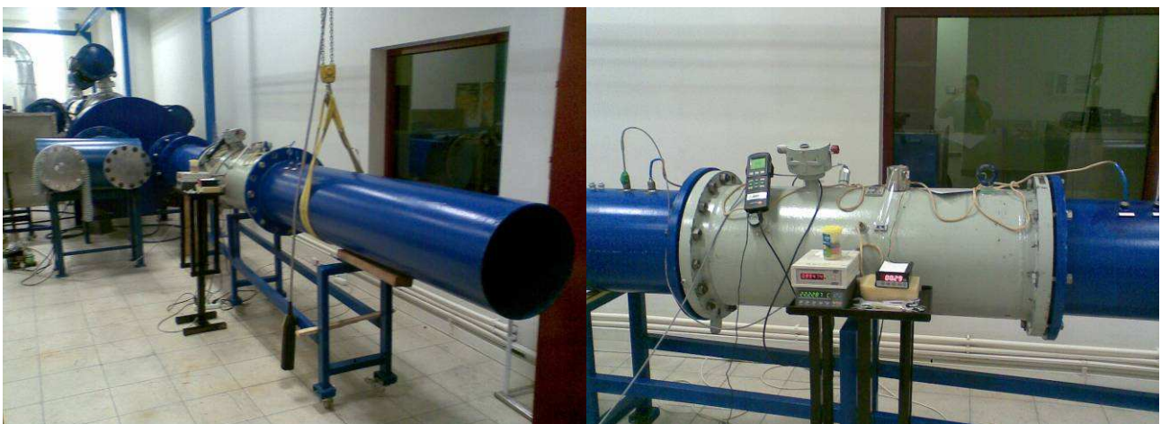
Figure 18 – Photograph of a tested meter on the line in UME
