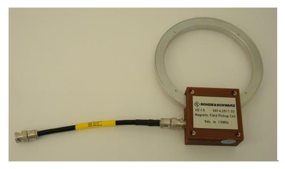
Frequency range: 5 Hz to 10 MHz. Connector type: BNC.
