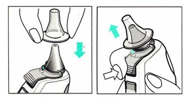
Figure 19: Attaching/detaching probe cover
