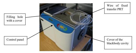
Figure 4: Transfer bath with the blackbody positioned on a level surface
