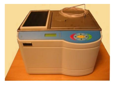
Figure 1: Transfer calibration bath with the EN-type of blackbody
