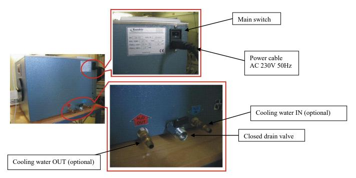
Figure 6: Back side of the transfer BB
