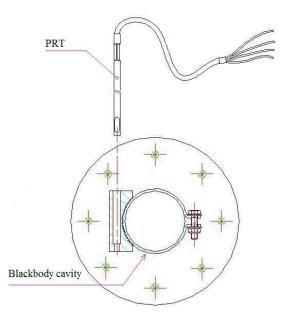
Figure 5: Position of the transfer PRT in the transfer BB
