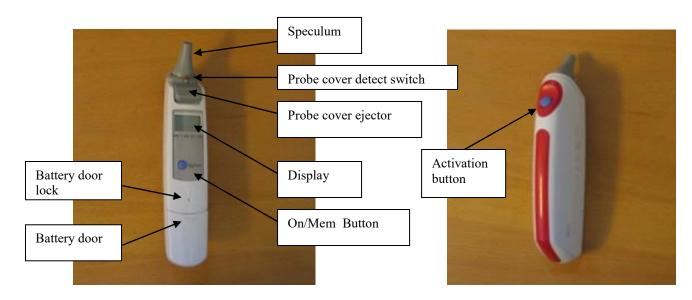
Figure 15: Transfer IRET; front and back view
