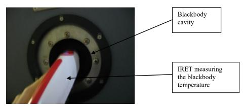
Figure 17: Measuring temperature of the blackbody
