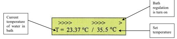
Figure 12: Regulation of water temperature in the bath
