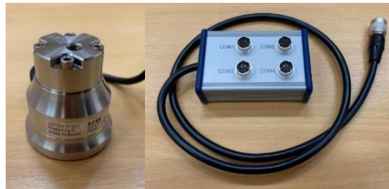
Figure 13 – CETONI pressure sensor (pressure range 0-5 bar) and I/O-splitter
