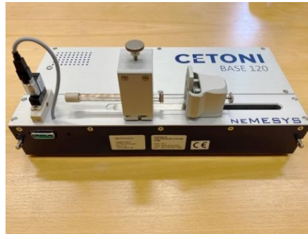
Figure 12 – Flow generator: Syringe pump CETONI Nemesys including glass syringe
