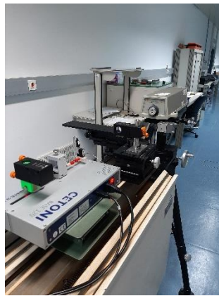
Figure 5 - Setup for the CETONI Nemesys pump calibration
