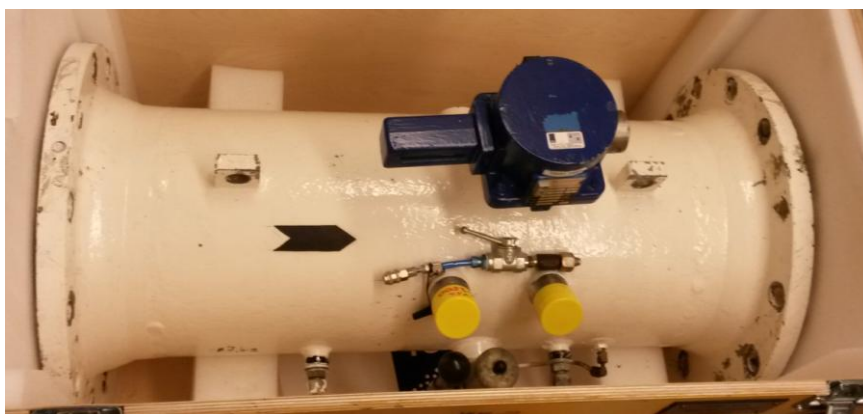
Figure 1 Instromet turbine meter G2500
