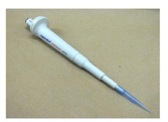
Figure 1- Fixed micropipette
