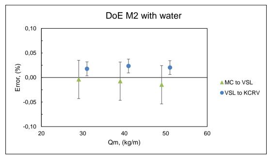
Figure 11: Meter 2 degree of equivalence with uncertainty. (Error bars represent worst case for all rates.)
