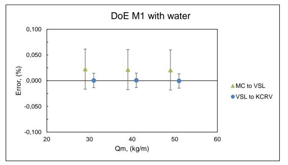
Figure 9: Meter 1 degree of equivalence with uncertainty. (Error bars represent worst case for all rates.)
