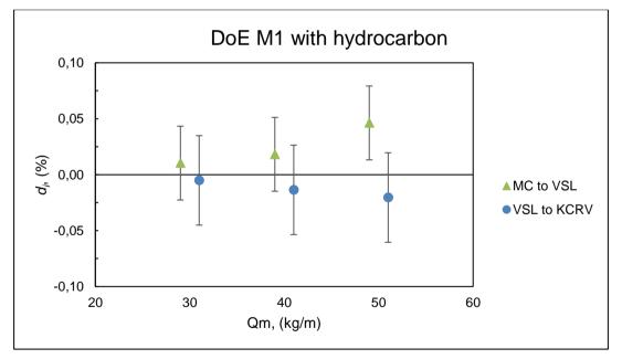
Figure 13: Meter 1 degree of equivalence with uncertainty. (Error bars represent worst case for all rates.)
