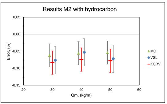
Figure 14: Meter 2 measurement error with uncertainty. (Error bars represent worst case for all rates.)
