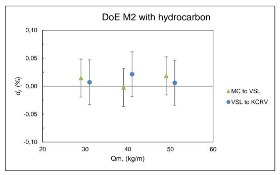
Figure 15: Meter 2 degree of equivalence with uncertainty. (Error bars represent worst case for all rates.)
