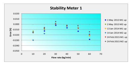
Figure 6: Meter 1 Test results to determine the stability of the transfer standards
