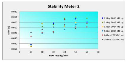
Figure 7: Meter 2 Test results to determine the stability of the transfer standards
