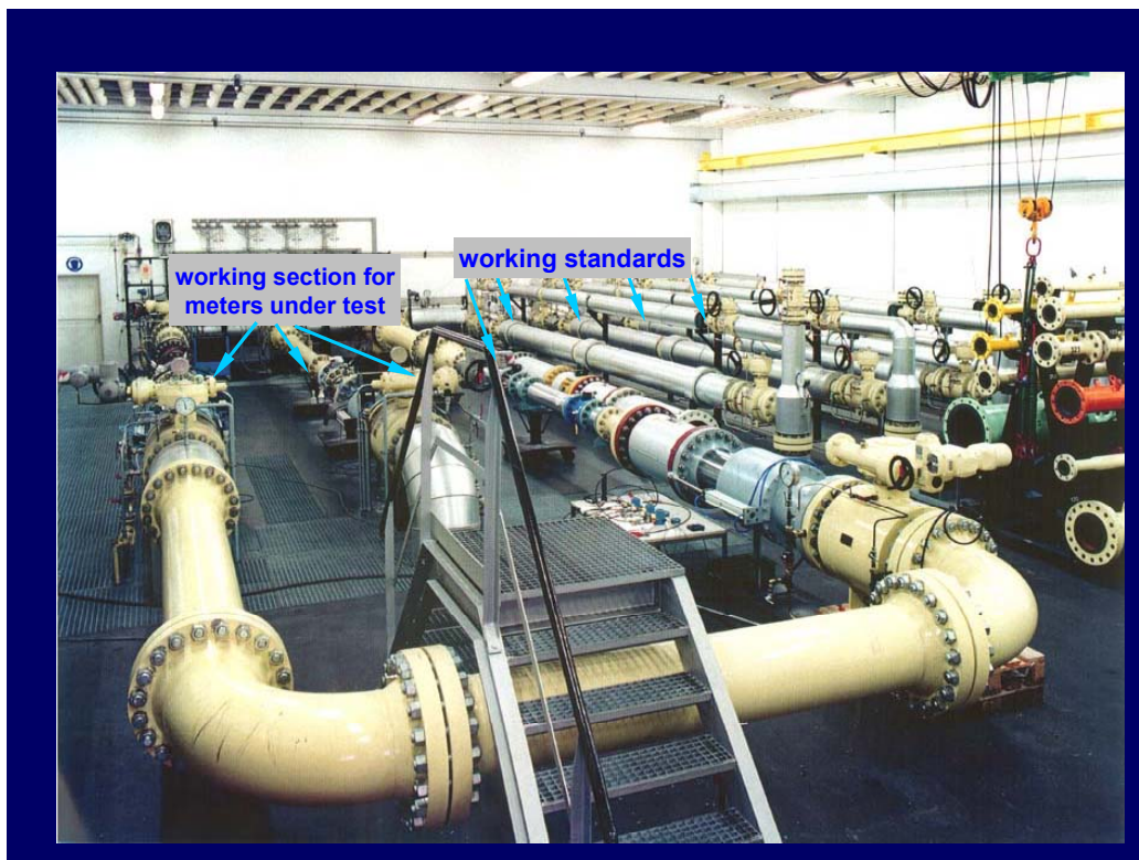
Figure 7: Outline of the national lab pigsar of PTB. In the right corner one recognizes the working standards which will be used to calibrate meters.
