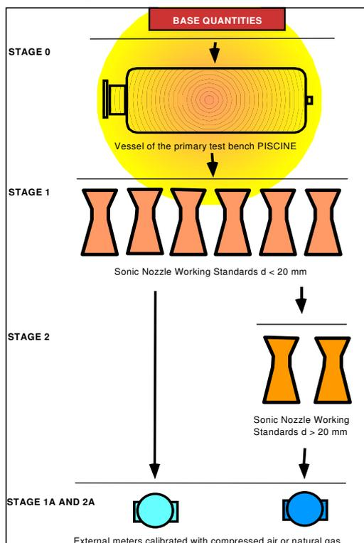
**Figure 5 The gas flow rate traceability chain**
