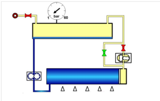
Figure 1 Gas Oil Piston Prover
