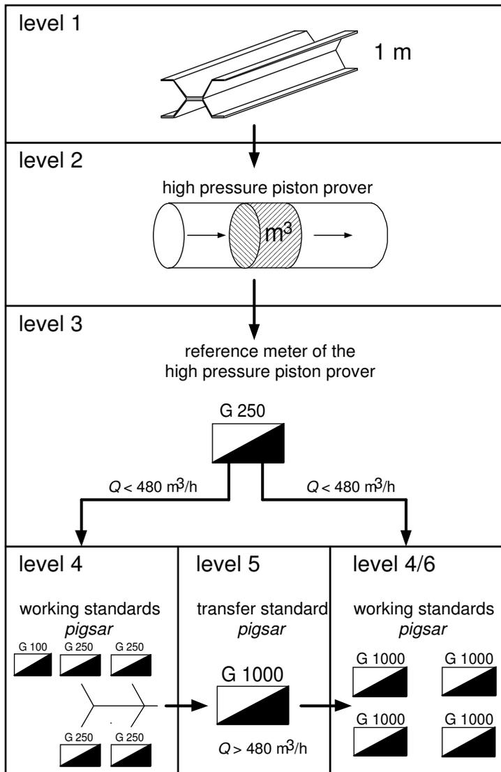
Figure 3 The high pressure traceability chain of *pigsar*
