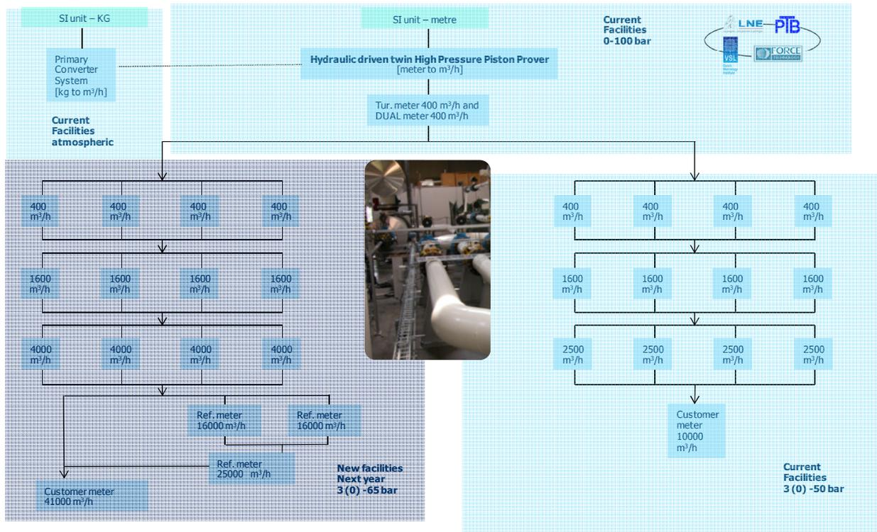
Figure 6 Traceability chain of FORCE
