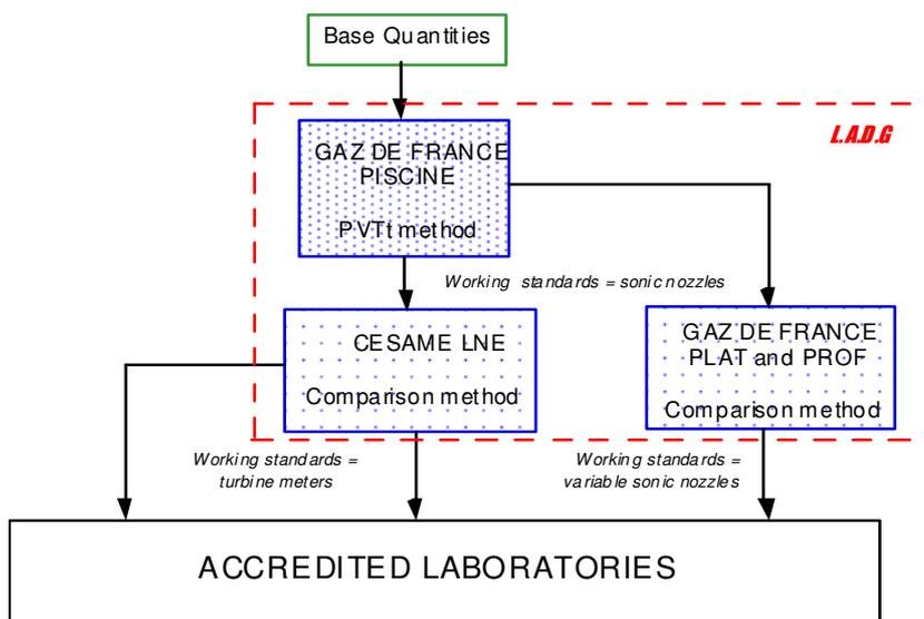
**Figure 4 Traceability chain of the French accredited laboratories for gas flow measurements**
