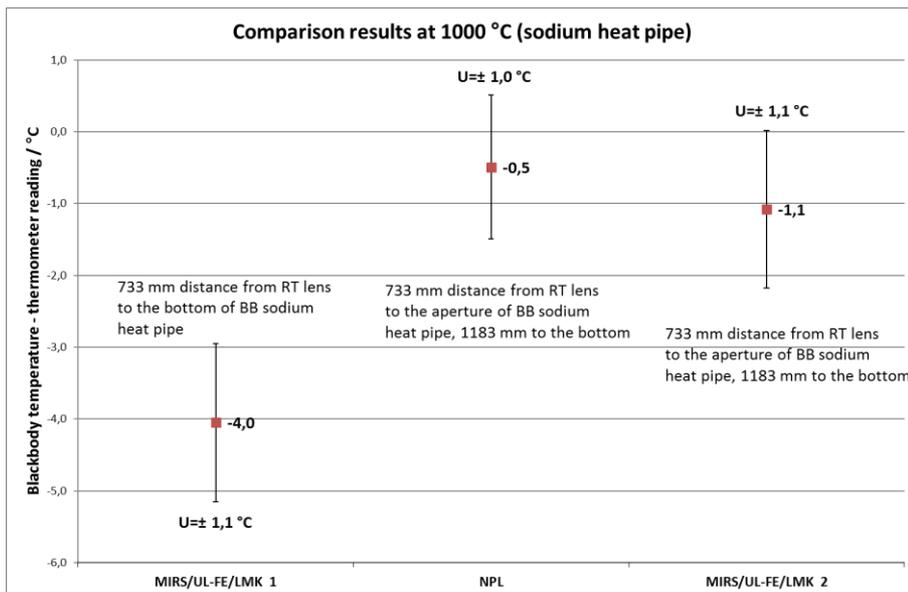
Figure 3: Results of comparison between MIRS/UL-FE/LMK and NPL at 1000 °C
