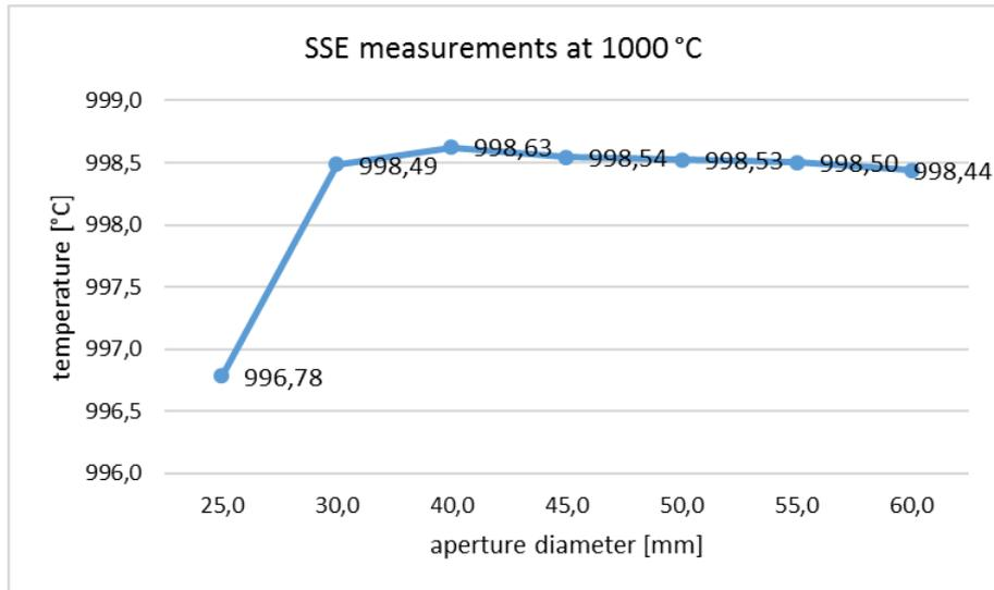
Figure 7: Results of SSE measurements at 1000 °C at a distance of 733 mm from the blackbody aperture
