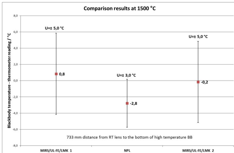
Figure 6: Results of comparison between MIRS/UL-FE/LMK and NPL at 1500 °C
