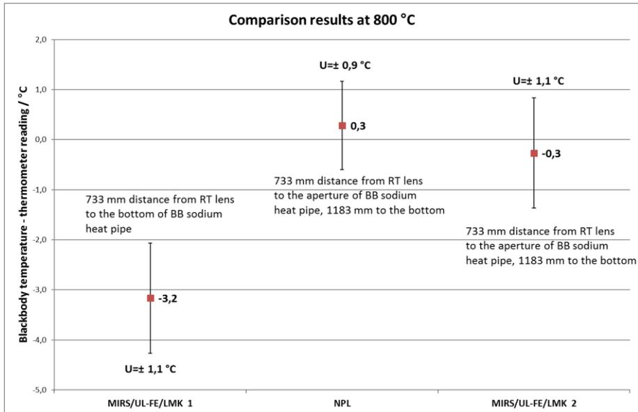
Figure 2: Results of comparison between MIRS/UL-FE/LMK and NPL at 800 °C
