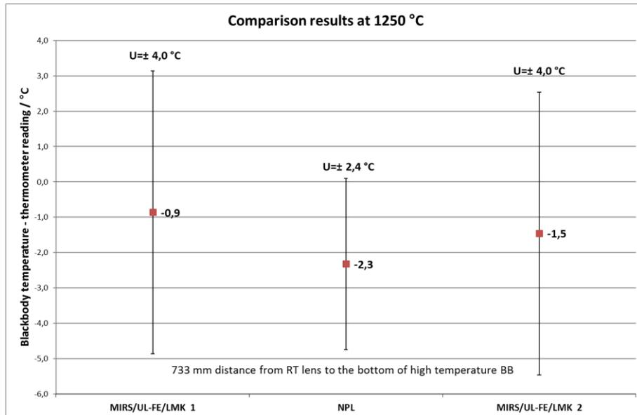
Figure 5: Results of comparison between MIRS/UL-FE/LMK and NPL at 1250 °C
