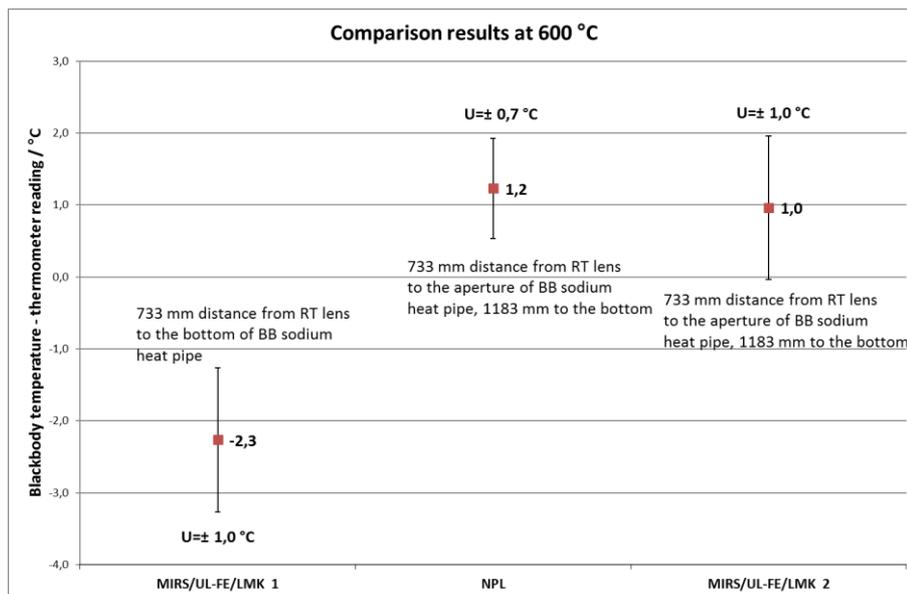
Figure 1: Results of comparison between MIRS/UL-FE/LMK and NPL at 600 °C
