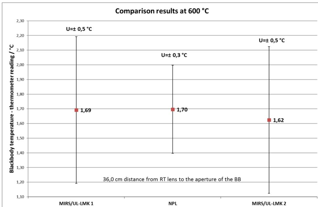
Figure 6: Results of comparison between MIRS/UL-FE/LMK and NPL at 600 °C
