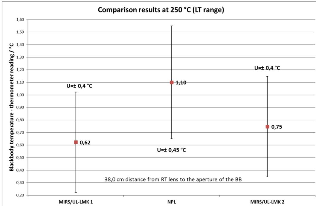
Figure 4: Results of comparison between MIRS/UL-FE/LMK and NPL at 250 °C (LT range)
