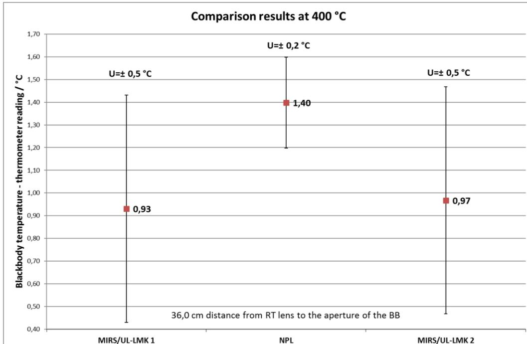
Figure 6: Results of comparison between MIRS/UL-FE/LMK and NPL at 400 °C
