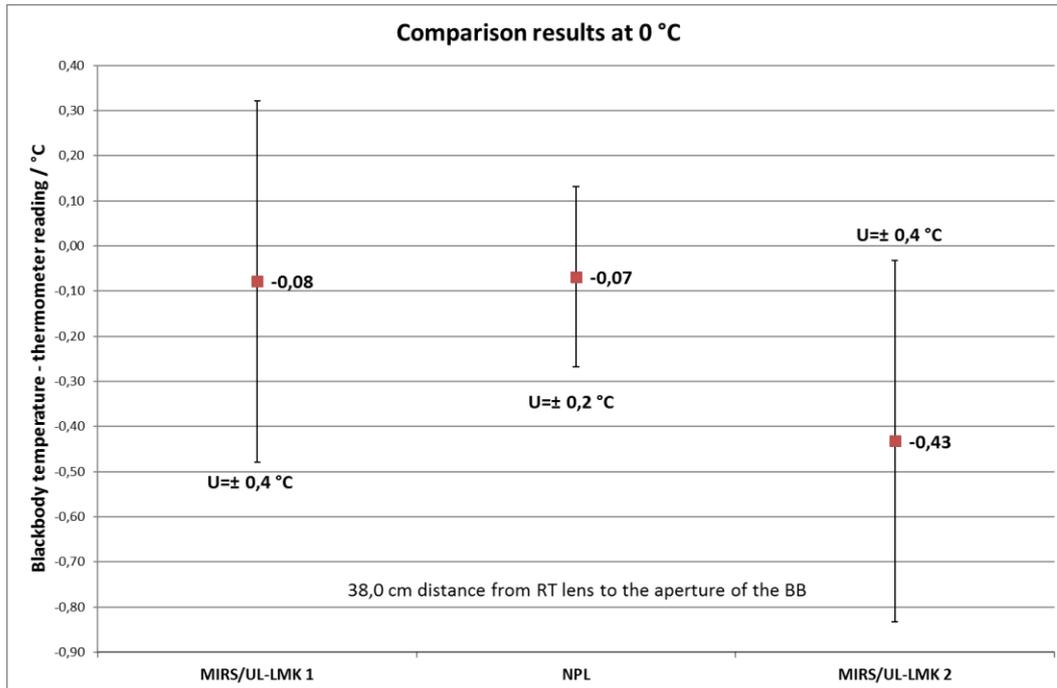
Figure 2: Results of comparison between MIRS/UL-FE/LMK and NPL at 0 °C
