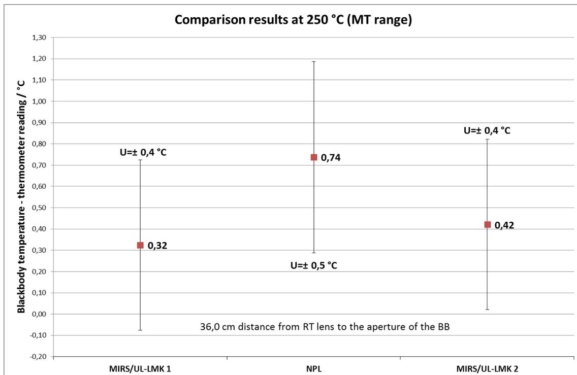
Figure 5: Results of comparison between MIRS/UL-FE/LMK and NPL at 250 °C (MT range)
