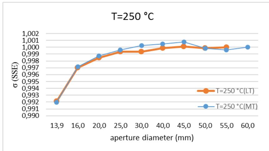
Figure 7: Results of SSE measurements at 250 °C
