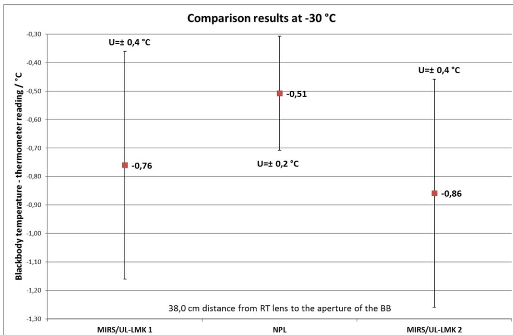
Figure 1: Results of comparison between MIRS/UL-FE/LMK and NPL at -30 °C
