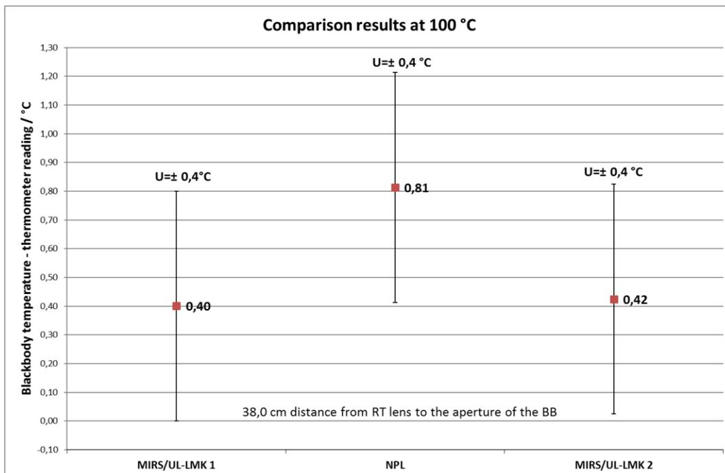
Figure 3: Results of comparison between MIRS/UL-FE/LMK and NPL at 100 °C
