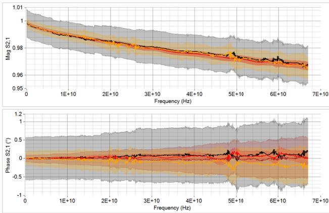
Fig. 2. Measurements of the male-female adaptor transmission coefficient. Refer to Fig 1 for the graph series legend. The top graph is magnitude and the bottom graph is phase with respect to the phase of the mean at each frequency.
