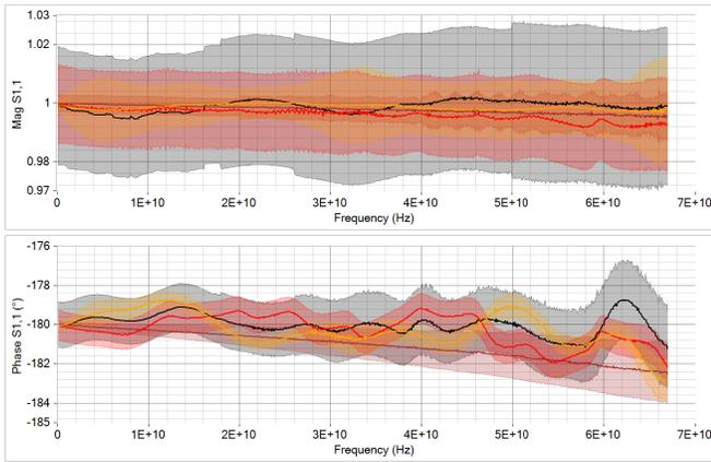
Fig. 1. Measurements of the female flush short-circuit device reflection coefficient. The black line shows LNE's results, the brown line METAS's results, the red line NPL's results and the orange line PTB's results. The top graph is magnitude and the bottom graph is phase.
