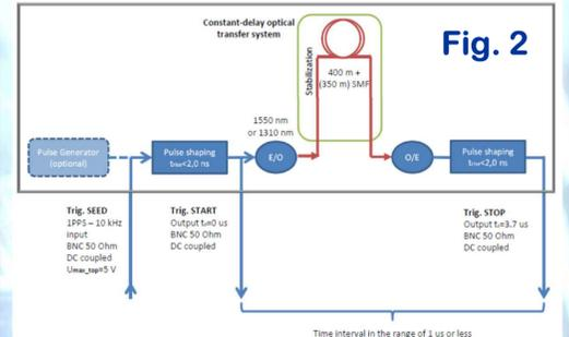
Fig. 2 The block scheme of operation of InLambda standards
