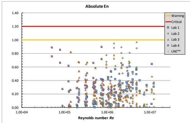
Figure 2:  $E_n$  [-] values versus  $Re$  number [-] with respect to HRV level. The yellow line is warning level corresponding to  $E_n = 1$ . The red line is the critical level corresponding to  $E_n = 1.2$ .
