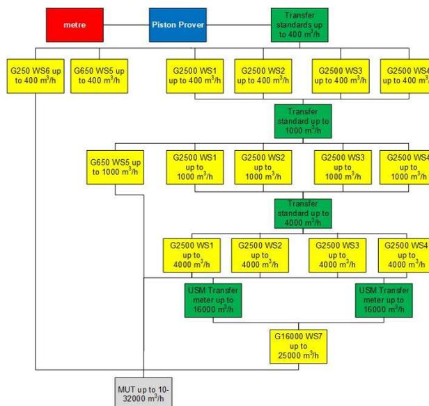
**Figure 4:** Schematic representation of the Danish traceability chain for high-pressure gas flow measurement. The reference meters (yellow) numbered WS1 .. WS7, are traceable via transfer standards (green) to the piston prover (blue) and the SI unit metre (red). The meter under test is calibrated by using a combination of reference meters.
