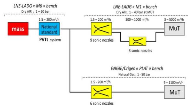
Figure 3: Schematic representation of the French traceability chain for high-pressure gas flow measurement. Sonic nozzles (yellow) are directly traceable PVTt system (blue), which is traceable to mass (red). The meter under test is calibrated by using a combination of sonic nozzles.
