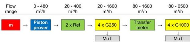
Figure 2: Schematic representation of the German traceability chain for high-pressure gas flow measurement. The reference meters (yellow) are traceable via transfer standards (green) to the piston prover (blue) and the SI unit metre (red). The meter under test (grey) is calibrated by using a combination of reference meters.
