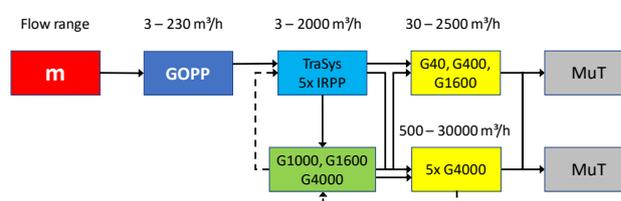
**Figure 1:** Schematic representation of the Dutch traceability chain for high-pressure gas flow measurement. The reference meters (yellow) are traceable via transfer standards (green) and TraSys (light blue) to the piston prover (blue) and the SI unit metre (red). The meter under test (grey) is calibrated by using a combination of reference meters. The dashed lines indicate the bootstrapping process which is used to calibrate the instrument beyond the range covered by a higher standard.
