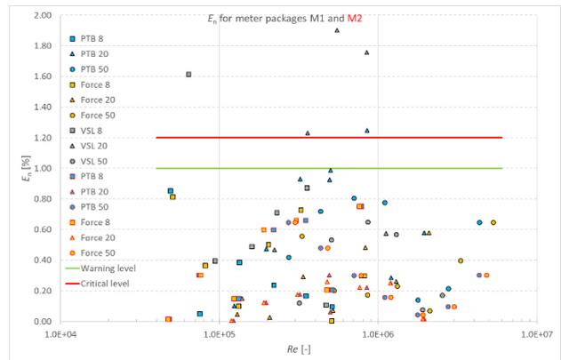
Figure 2:  $E_n$  [-] values versus  $Re$  number [-]. The green horizontal line is the warning level corresponding to  $E_n=1$ . The horizontal red line is the critical level corresponding to  $E_n=1.2$ .
