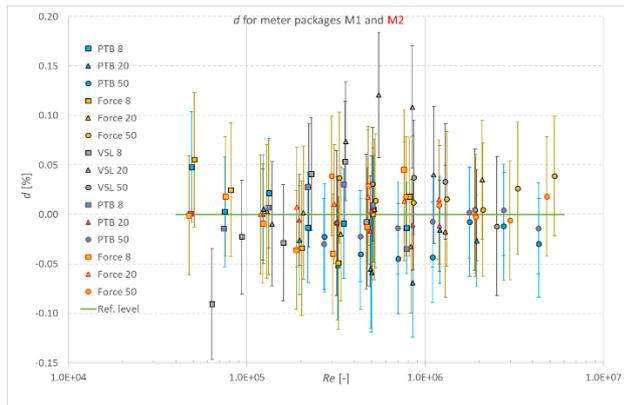
Figure 1: Deviations  $d$  [%] versus the Reynolds number  $Re$  [-]. The markers for meter M1 have a black outline and the markers for meter M2 a red outline. The symbol colors correspond to the participating laboratory and the symbol shapes to the calibration pressure. The horizontal green line is the reference level  $d=0$ .
