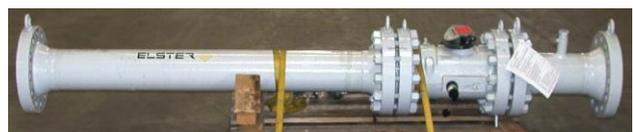
Figure 3: One of the 4" packages used for the piston prover intercomparison.
